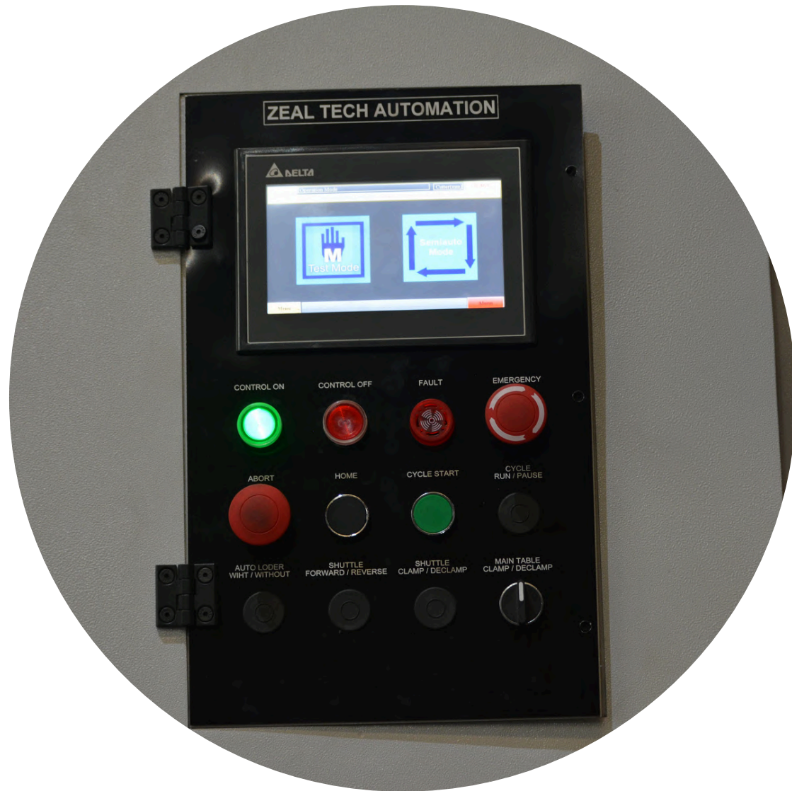
Operator- friendly Delta Touch Screen HMI with Diagnosis.
